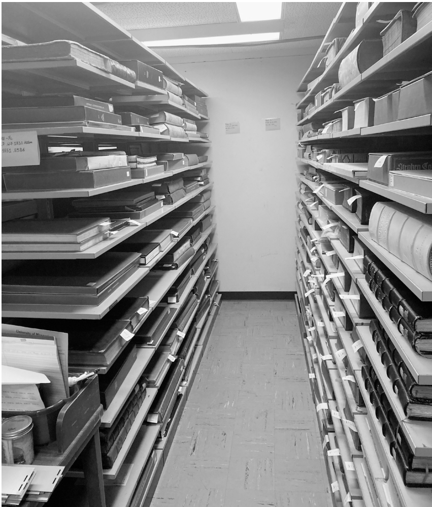
This photograph shows a row of Rare-XL shelving after the project was completed. The shelves at left are set with 19cm spacing and at right with 14cm intervals. Oversize books are shelved with no more than two volumes on any shelf.
