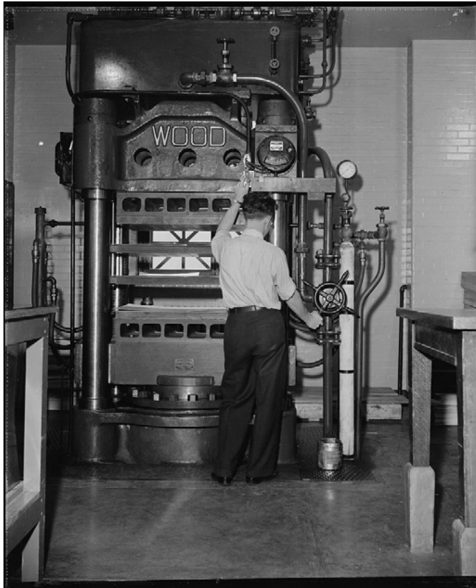
ILLUSTRATION 2. “National Archives. Washington, D.C., Nov. 22 [1939]. In the powerful press, the sheets of acetate, under heat and pressure ‘melt’ into the pores of the paper and adhere to each other as well...” (Harris & Ewing collection, Library of Congress Prints & Photographs Division)
